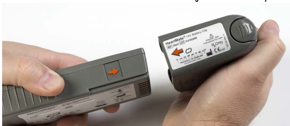
Figure 61 Insert Battery into Battery Clip
