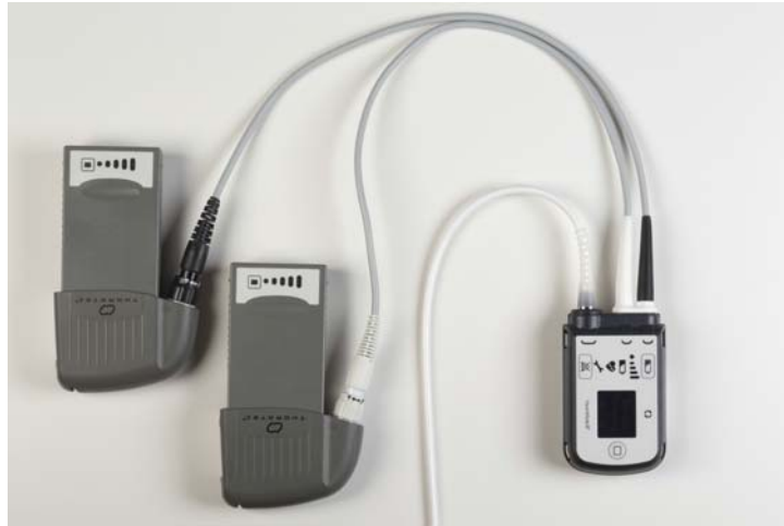
Figure 64 System Controller Connected to Batteries
