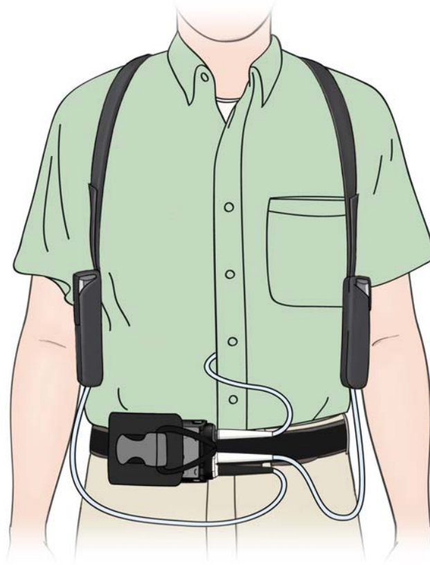
Figure 129 Belt Attachment Used with Battery Holster
