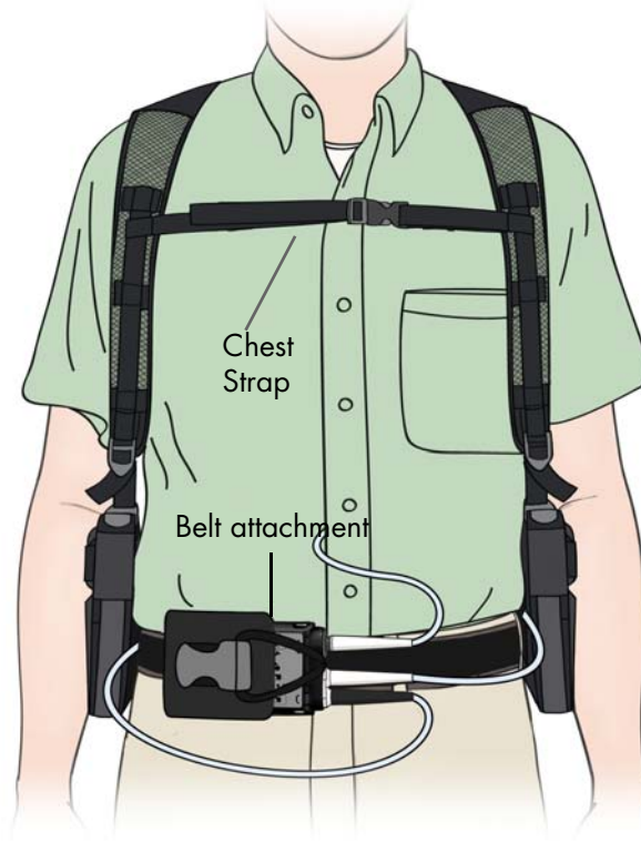
Figure 134 Holster Vest with Belt Attachment and Shoulder Strap
