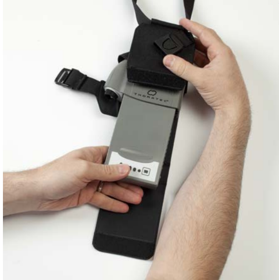
Figure 137 Insert Battery and Battery Clip Into Holster
