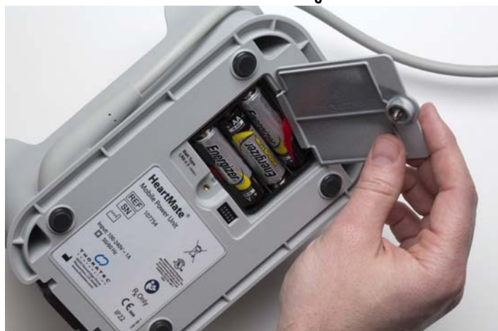
Figure 40 Remove the Battery Compartment Cover
