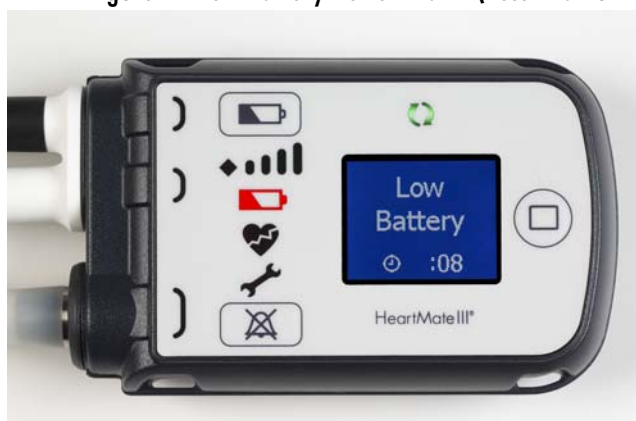
Figure 21 Low Battery Power Alarm (Less Than 5 Minutes of Power Remain)
