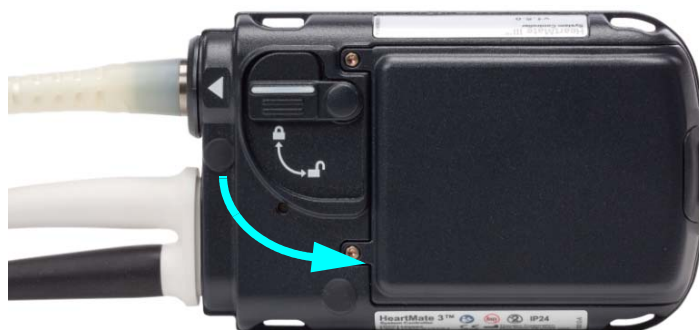
Figure 34 Unlock the Safety Lock
