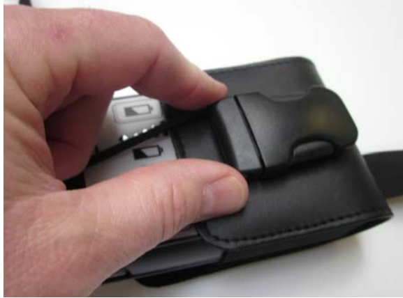
Figure 111 Clip the Strap Into Place so the System Controller is Secure
