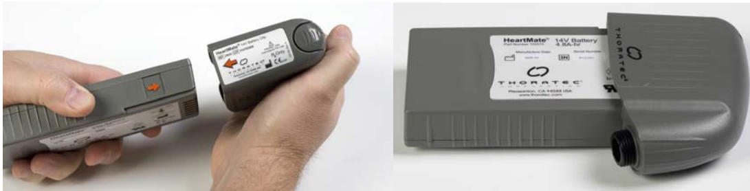
Figure 66 Align Orange Arrows and then Insert Battery into Battery Clip
