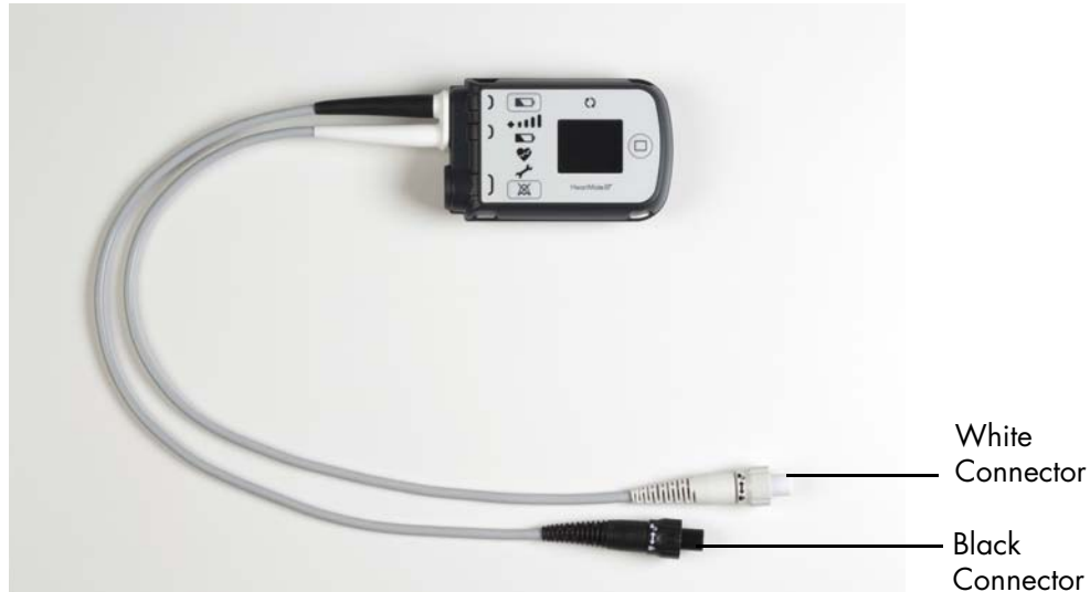
Figure 62 System Controller Power Cables with Black and White Connectors
