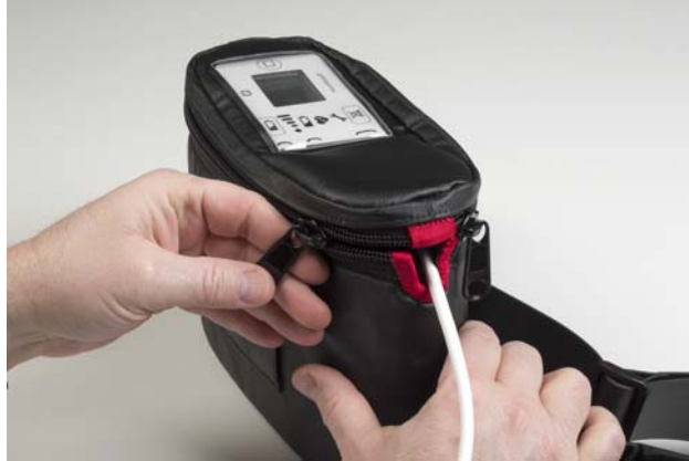
Figure 94 Carefully Close the Shower Bag so the Driveline Exits the Bag through the Protective Red Tabs
