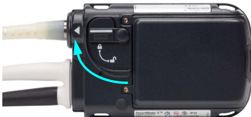
Figure 12 Insert and Lock the Driveline Into the Socket
