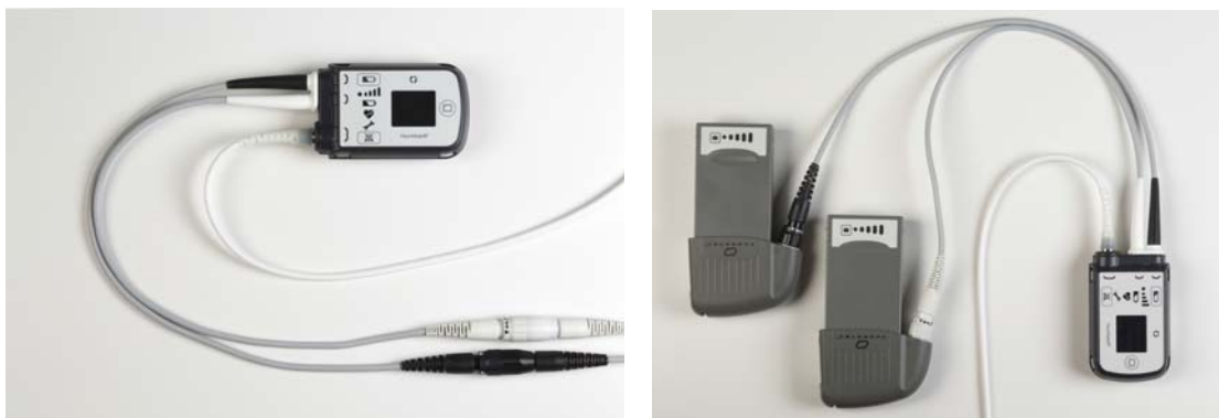
Figure 22 System Controller in Run Mode While Connected to the Mobile Power Unit (left) and to Batteries (right)
