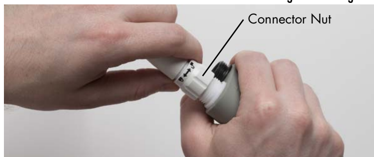
Figure 147 Tighten the Connector Nut
