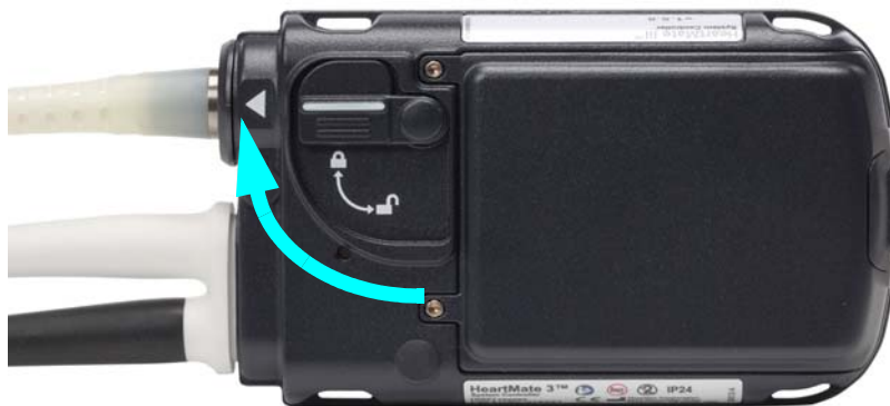
Figure 33 Closing the Safety Lock
