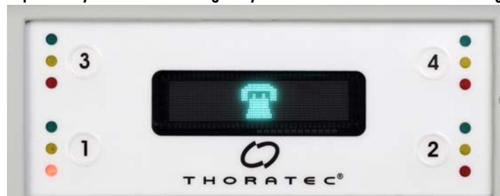
Figure 145 Telephone Symbol and Red Light by Pocket 1 Indicate that the Charger Detects a Problem
