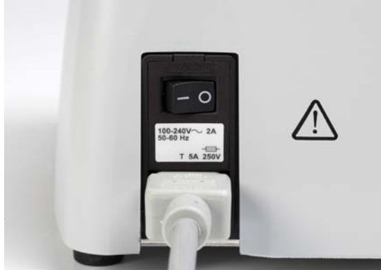
Figure 70 Plug the Power Cord into the Rear of the Battery Charger
