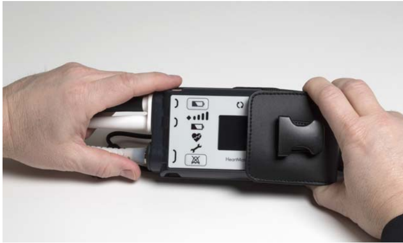
Figure 109 Slide the System Controller Into the Belt Attachment
