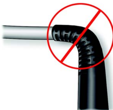
Figure 16 Do Not Sharply Bend the Power Cables
