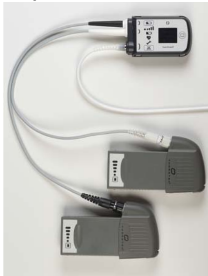
Figure 115 Make Sure the Power Cables and Driveline are Not Twisted
