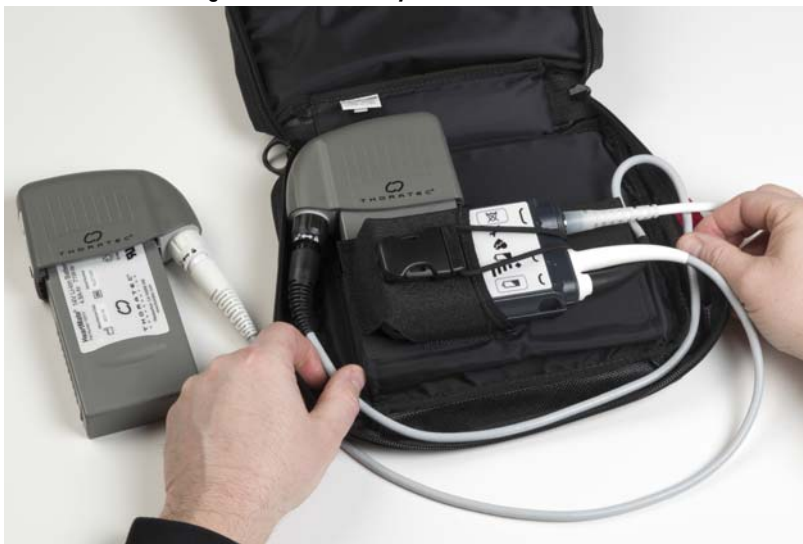
Figure 119 Carefully Position the Power Cable Around the Edge of the Bag
