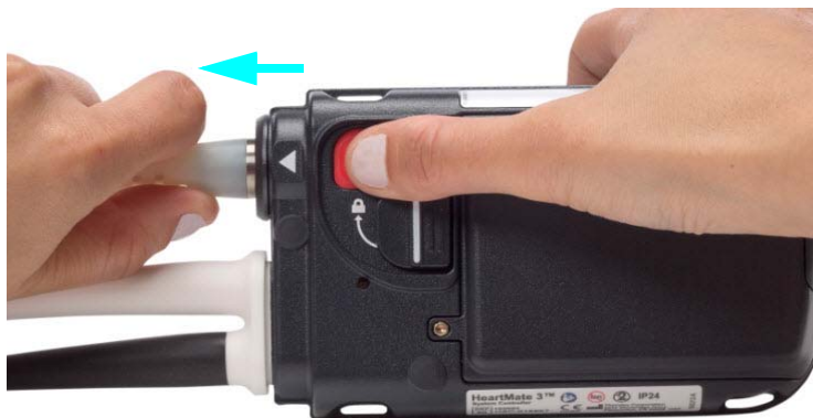
Figure 35 Grasp the Metal End and Remove the Driveline
