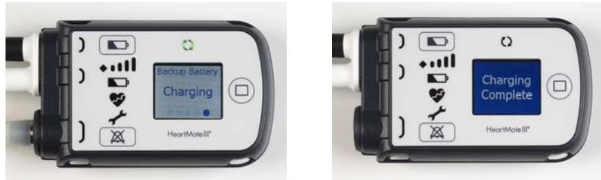
Figure 27 System Controller Charging or Charging Complete
