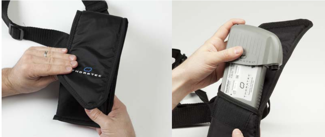
Figure 131 Open VELCRO Flap and Insert Battery with Attached Battery Clip
