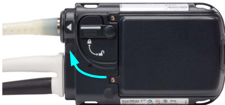
Figure 37 Closing the Safety Lock
