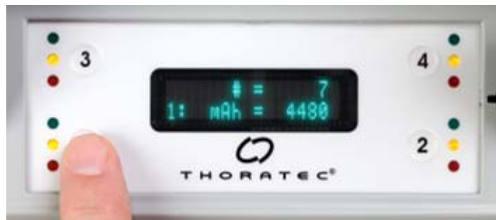
Figure 78 Press the Button a Second Time to Display Battery Charge Cycle Information
