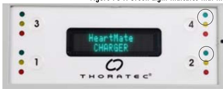
Figure 75 A Green Light Indicates that the Battery is Charged
