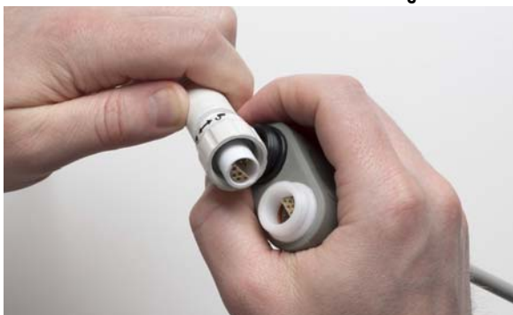
Figure 49 Carefully Align the Connectors
