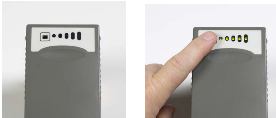
Figure 60 Press the Power Gauge Button to Check the Battery Charge Level
