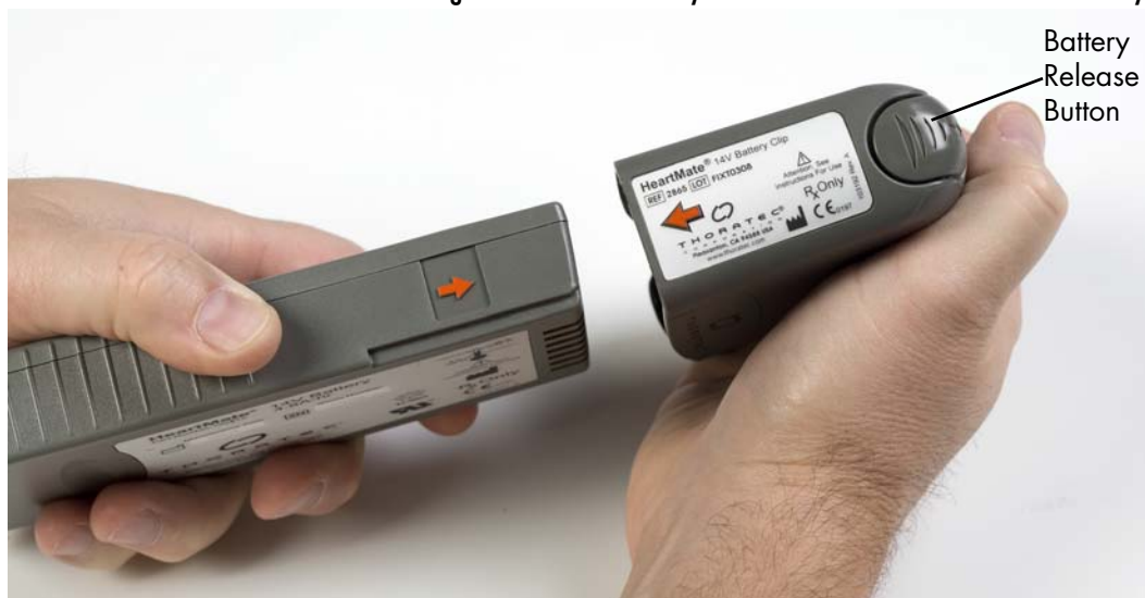
Figure 59 Press Battery Release Button and Withdraw Battery
