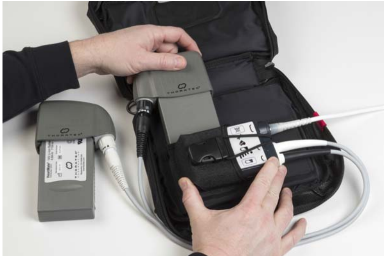
Figure 118 Place Battery and Attached Battery Clip into Consolidated Bag
