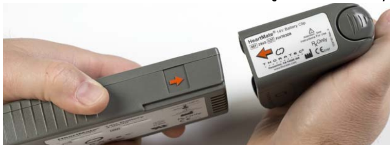
Figure 67 Insert Battery into Battery Clip
