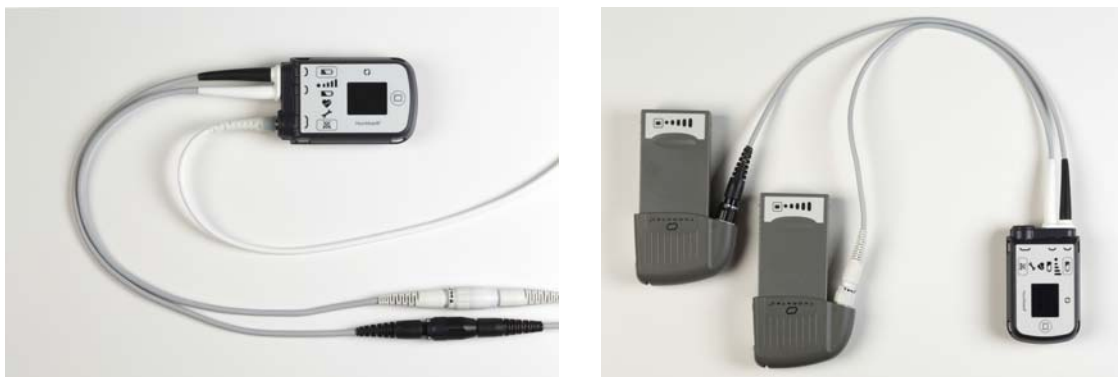
Figure 26 System Controller on Mobile Power Unit Power (left) and Battery Power (right)
