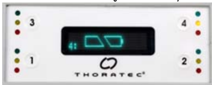
Figure 80 The Battery in Pocket 4 is Being Calibrated
