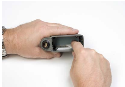
Figure 148 Clean the Contacts on the Batteries and Battery Clips
