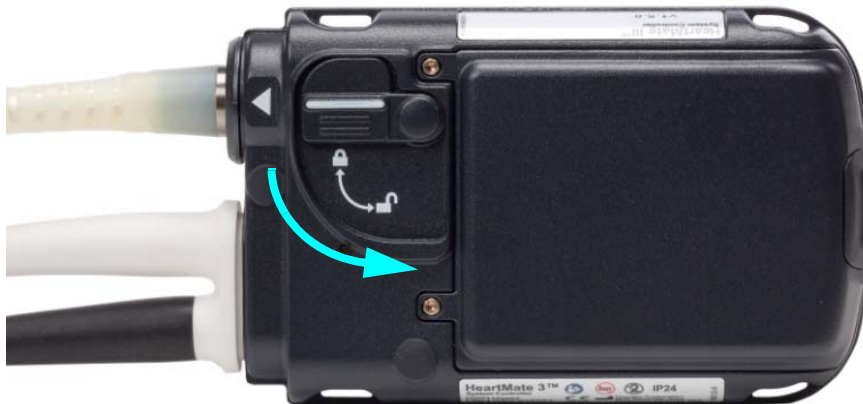
Figure 13 Unlock the Safety Lock
