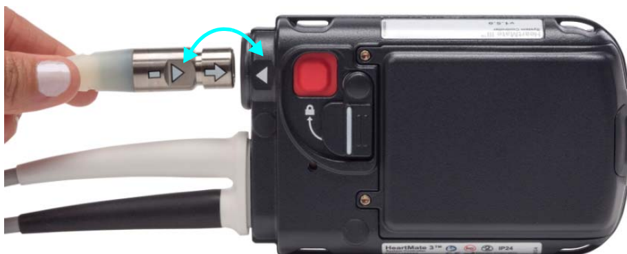
Figure 11 Align the Arrows
