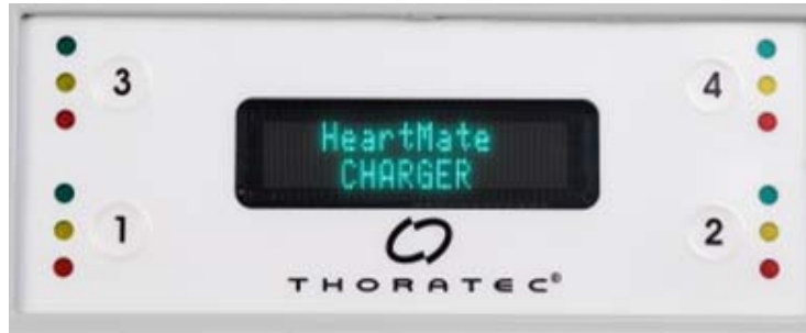
Figure 72 The Battery Charger is Ready to Use
