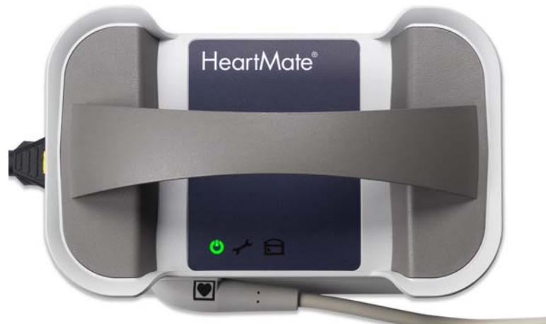
Figure 144 Indicators on the Mobile Power Unit
