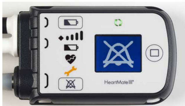
Figure 143 Alarm Silence Indicator
