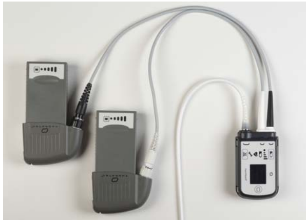
Figure 88 Make Sure the Power Cables and Driveline are Not Twisted
