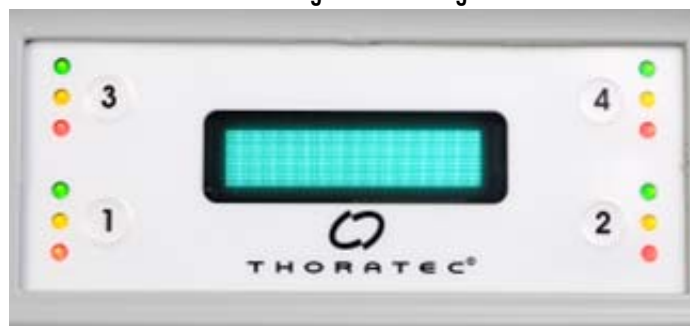
Figure 71 All Lights Turn On When the Charger is Turned On
