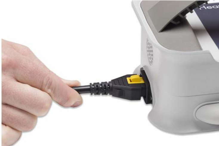
Figure 44 Pull Back to Ensure Secure Connection
