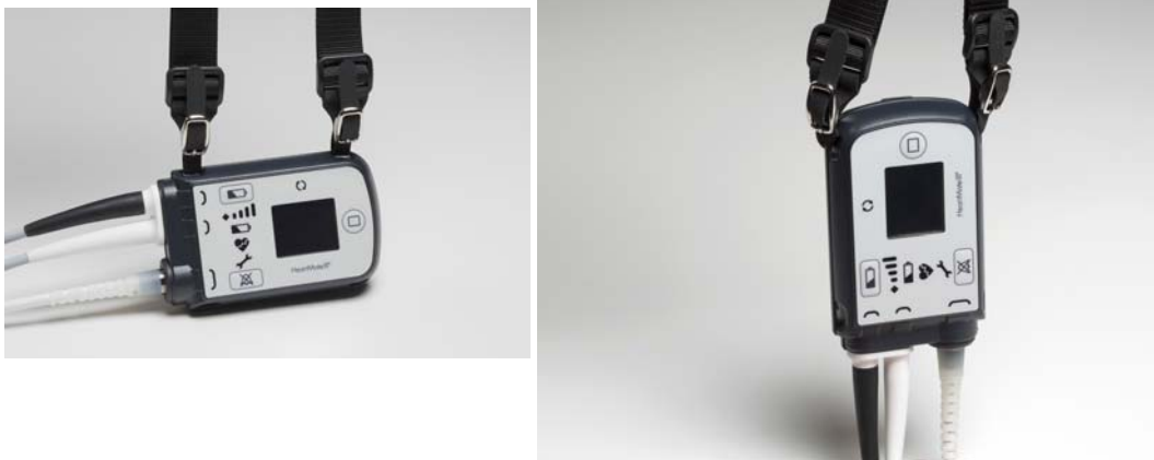
Figure 101 System Controller Suspended Horizontally (left) and Vertically (right) from Neck Strap
