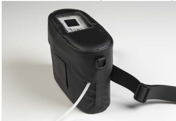
Figure 95 The Driveline Exiting a Closed Shower Bag
