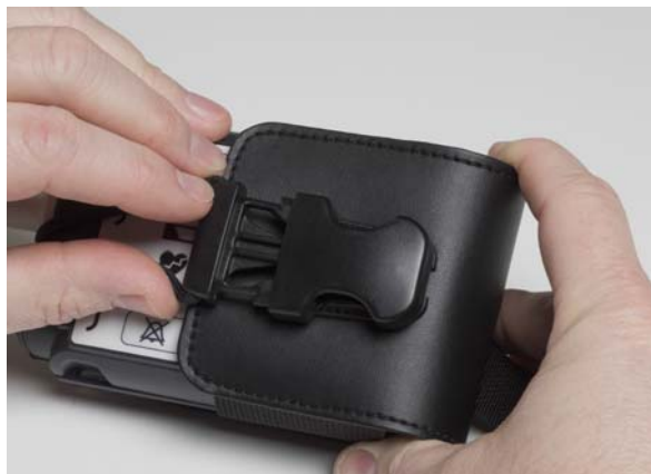
Figure 110 Place the Strap Between the Connectors
