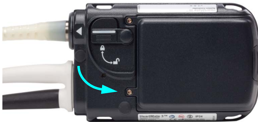
Figure 30 Unlock the Safety Lock
