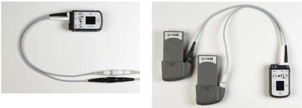
Figure 24 System Controller in Charge Mode on Mobile Power Unit Power (left) and Using Fully-Charged HeartMate Batteries (right)
